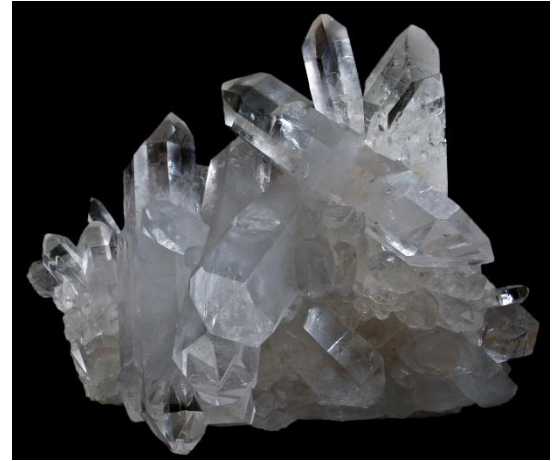
Crystalline solids such as this quartz have a very orderly structure.
