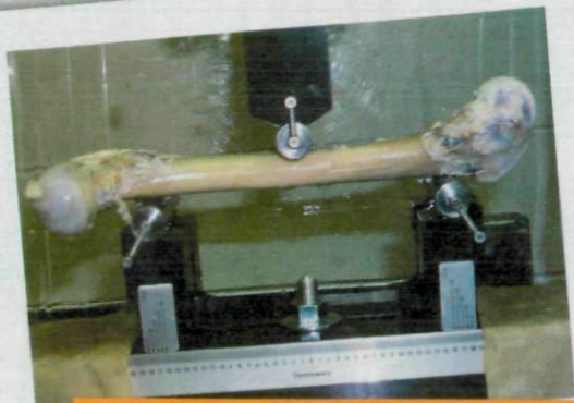
STRENGTH TEST: Under pressure, leg bones from hibernating and non-hibernating bears prove to be equally strong.
